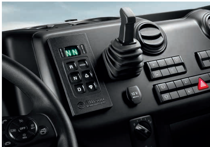
Greater comfort: automatic gear changes and convenient activation of power take-off with the Allison automatic transmission.
