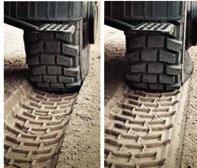
The principle of single tyres: the rear wheels follow in the tracks made by the front wheels. This improves traction and spares the terrain.
