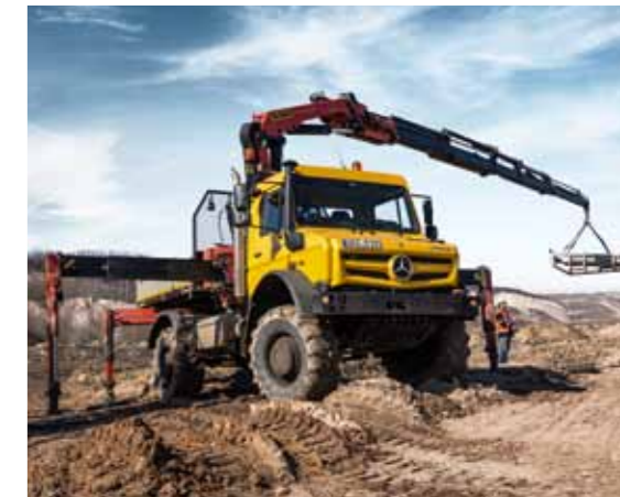
Off-road working made possible by engine and transmission-driven power take-offs.
