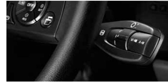
The right level of gear reduction at the touch of a button: convenient gear-changing with the steering-column switch.
