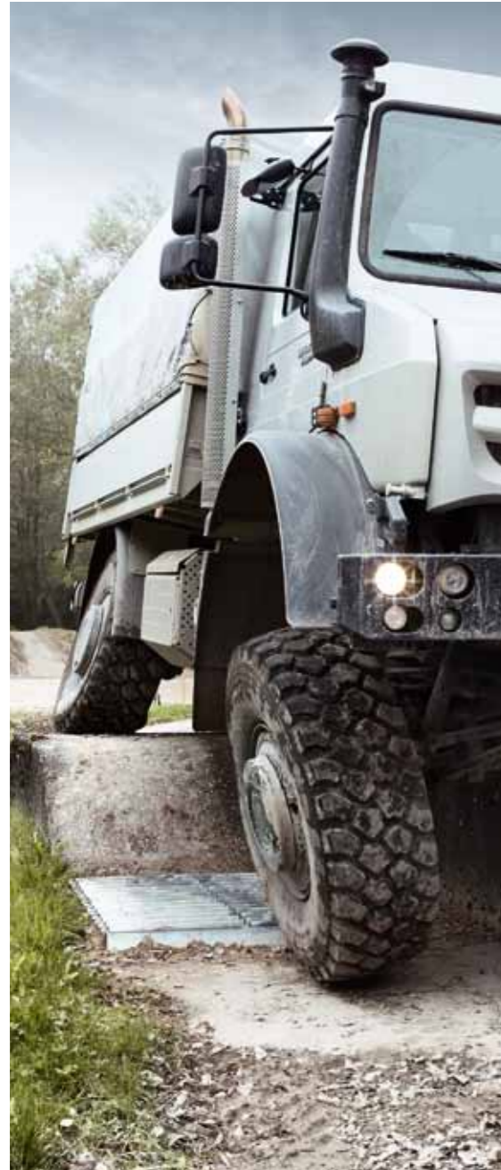
The offset frame with welded tubular cross members is the key to the vehicle's torsional flexibility.
