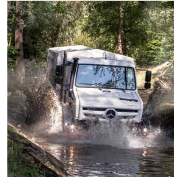
Water-resistant: high ground clearance, a vertical air-intake pipe and protected assemblies allow the Unimog to ford water depths of up to 80 cm (optional 120 cm).
