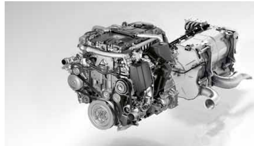
Increased output, lower emissions: the BlueTec 6 engine in the extreme all-terrain Unimog is a 4-cylinder unit with an output of 170 kW. Working in conjunction with the engine cooling system and the exhaust gas aftertreatment unit, this state-of-the-art engine complies with the Euro VI emissions standard. The standard requires a reduction of diesel particulates and nitrogen oxide emissions of 90% in comparison with Euro V.
