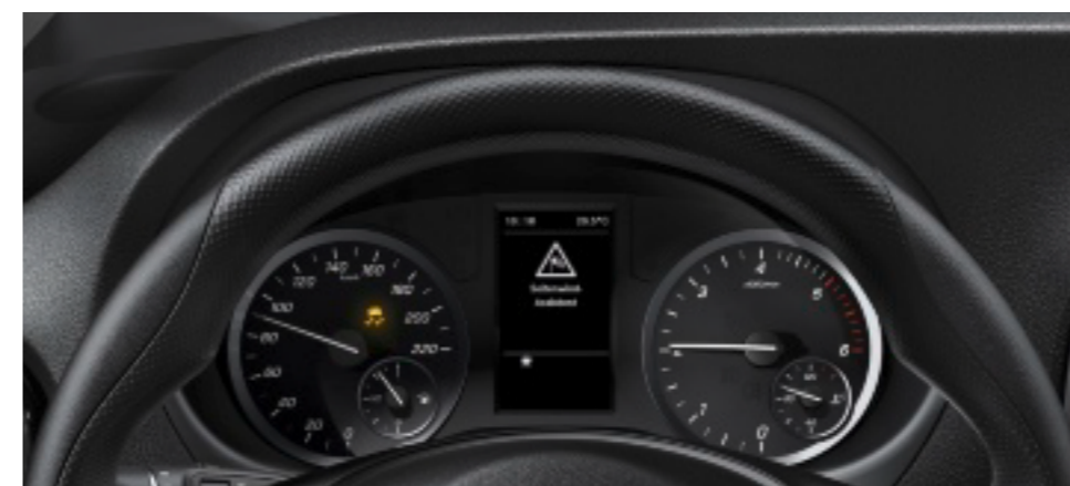
Crosswind Assist can reduce swerving caused by wind gusts with braking interventions on the upwind wheels.
