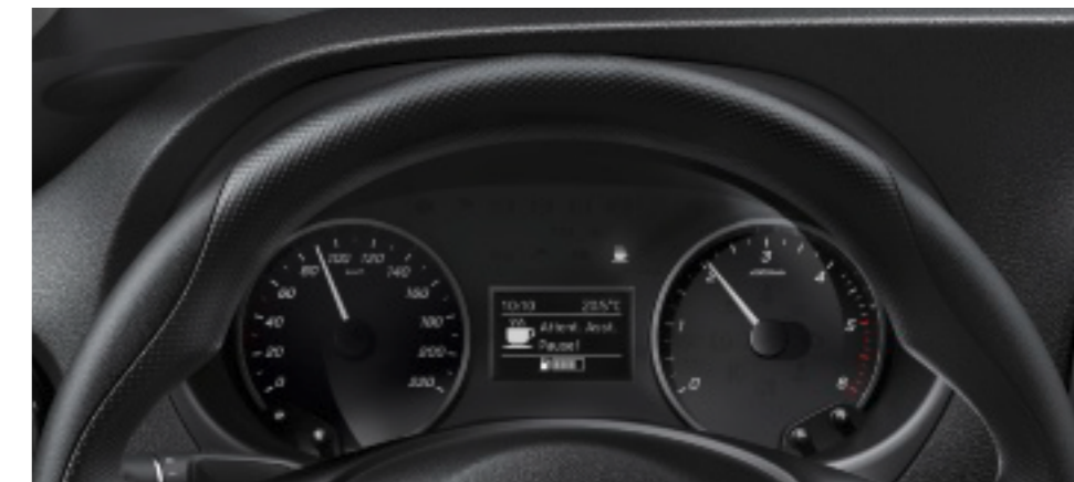
The ATTENTION ASSIST system can help to recognise signs of fatigue and therefore provides you with increased safety, particularly when driving at night and on long journeys.
