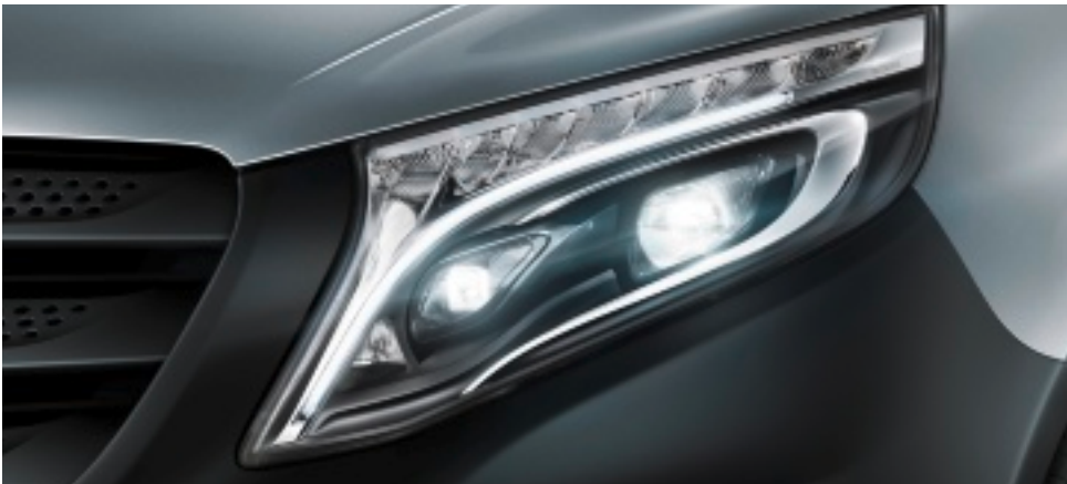
The LED Intelligent Light System improves the vision of the driver and therefore driving safety, as it can automatically adjust the illumination of the road surface to various driving conditions. Standard on 119 models. Optional on all other models.
