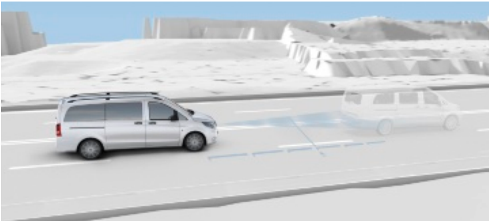
Active Distance Assist DISTRONIC can automatically maintain a safe distance to the vehicle travelling in front and thus relieves strain on the driver, for example in stop-and-go traffic. Standard on 119 models. Optional on other models.
