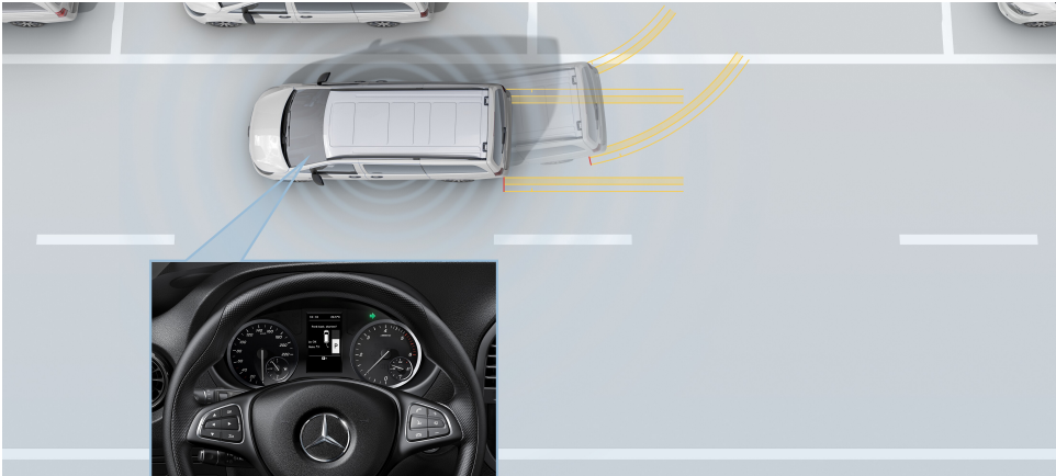
The Active Parking Assist feature can detect parking spaces and supports with active steering interventions when parking in longitudinal or lateral parking spaces. Optional on all 111 models.
