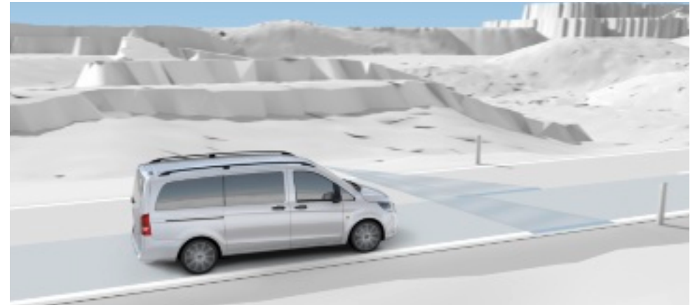
The Blind Spot Assist (visual and audible warning) and Lane Keeping Assist (haptic and audible warnings) can help the driver stay in lane or change lanes on multi-lane roads.
