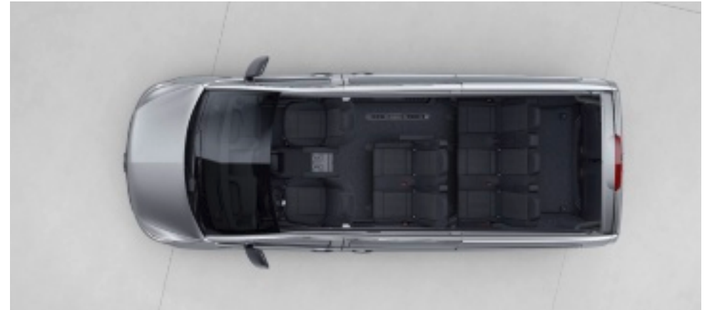
The guide rail system with quick-release attachment system allows more variable positioning of the seats and bench seats and additionally helps to secure luggage and/or load.
